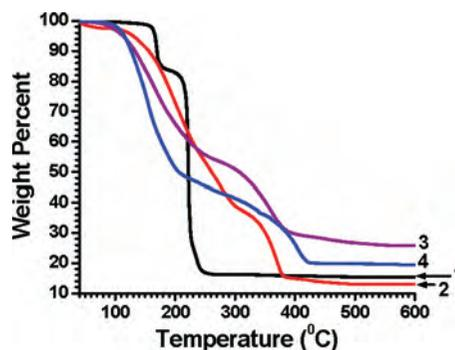
**Figure 5.** Atmospheric pressure thermogravimetric analysis (TGA) of the volatility characteristics of complexes **1–4**. The weight loss data were recorded at a ramp rate of 2.5 °Cmin<sup>−1</sup> and 50 mL min<sup>−1</sup> N<sub>2</sub> flow rate.
