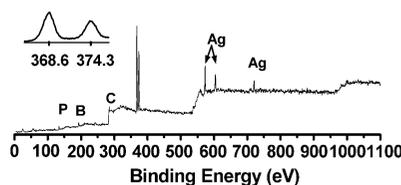
**Figure 11.** XPS spectrum of a Ag film deposited on 52100 steel by AACVD using precursor **2**. Peaks are labeled with their corresponding element. The inset is enlarged portion of the spectrum showing the Ag  $3d_{5/2}$  and  $3d_{3/2}$  ionizations.
