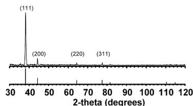
**Figure 10.** Glancing XRD  $\theta$ - $2\theta$  scan ( $\alpha = 0.30^\circ$ ) of Ag film grown on 52100 steel by AACVD using precursor **2**. Plotted underneath are the peak positions and relative intensities for the powder pattern of cubic phase Ag (PDF 04-0783).
