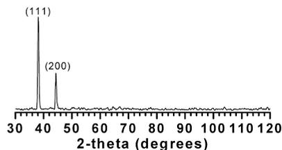
**Figure 6.** Glancing X-ray diffraction (GXR)  $\theta$ - $2\theta$  scan ( $\alpha = 0.30^\circ$ ) of a Ag film grown on MgO(100) by AACVD using precursor **1**. Peaks are labeled with the corresponding (*hkl*) reflections from cubic phase Ag (PDF 04-0783).
