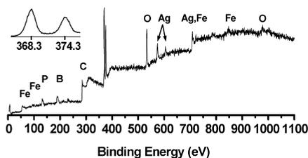
**Figure 7.** X-ray photoelectron spectroscopy (XPS) spectrum of a Ag film deposited on 52100 steel by AACVD using precursor **1**. Peaks are labeled with their corresponding element. The inset is enlarged portion of the spectrum showing the Ag  $3d_{5/2}$  and  $3d_{3/2}$  ionizations.
