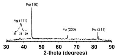
**Figure 9.** X-ray diffraction (XRD)  $\theta$ - $2\theta$  scan of Ag film grown on 52100 steel by AACVD using precursor **2**. Peaks are labeled with the corresponding (*hkl*) reflections from cubic phase Fe (PDF 06-0696) and cubic phase Ag (PDF 04-0783).
