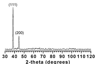
**Figure 8.** Glancing X-ray diffraction (GXR)  $\theta$ - $2\theta$  scan ( $\alpha = 0.30^\circ$ ) of Ag film grown on MgO(100) by AACVD using precursor **2**. Peaks are labeled with the corresponding (*hkl*) reflections for cubic phase Ag (PDF 04-0783).
